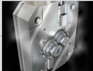
Casting, Die-casting 842 to 2462°F (450 to 1350°C)
