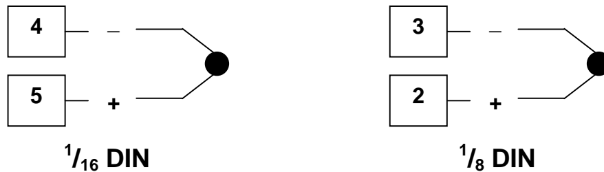
Figure 15. Thermocouple Input Connections
